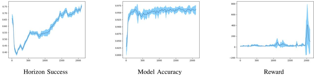
Fig. 6: The learning curves and uncertainty of the final policy trained over 14 hours when  $H = 16$  inside the “Enclosed Hallway” world. Performance over the horizon gets better as more data is collected to improve the model. From left to right, all plotted as a function of number of iterations: the probability of not colliding over the horizon (actor loss), the accuracy of the model predictions (critic loss), and the reward (performance on actual task).
