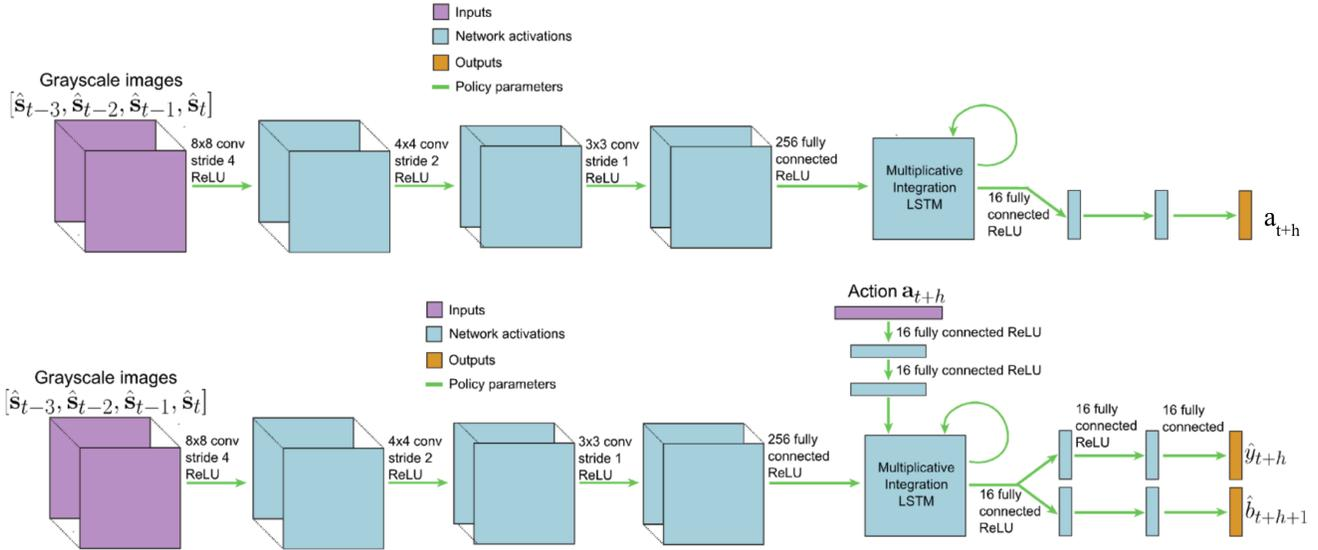
Fig. 5: The structure of the actor and critic networks.
